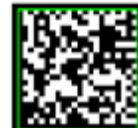
Quiet zone violation
