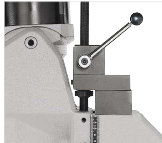
Height adjustment Fast, accurate setting of the work height.
